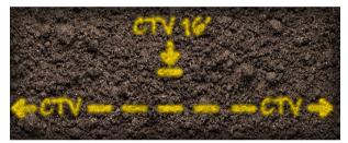
In areas where cables are **spliced**, the facilities should be located individually as far as possible on both sides of the splice. When the signal is distorted due to the near proximity to the splice a circle with "SP" should indicate the area of distortion or "splice pit".
