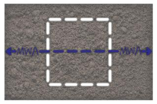
Dead ends, stub-outs, termination points, etc., shall be marked as follows:
